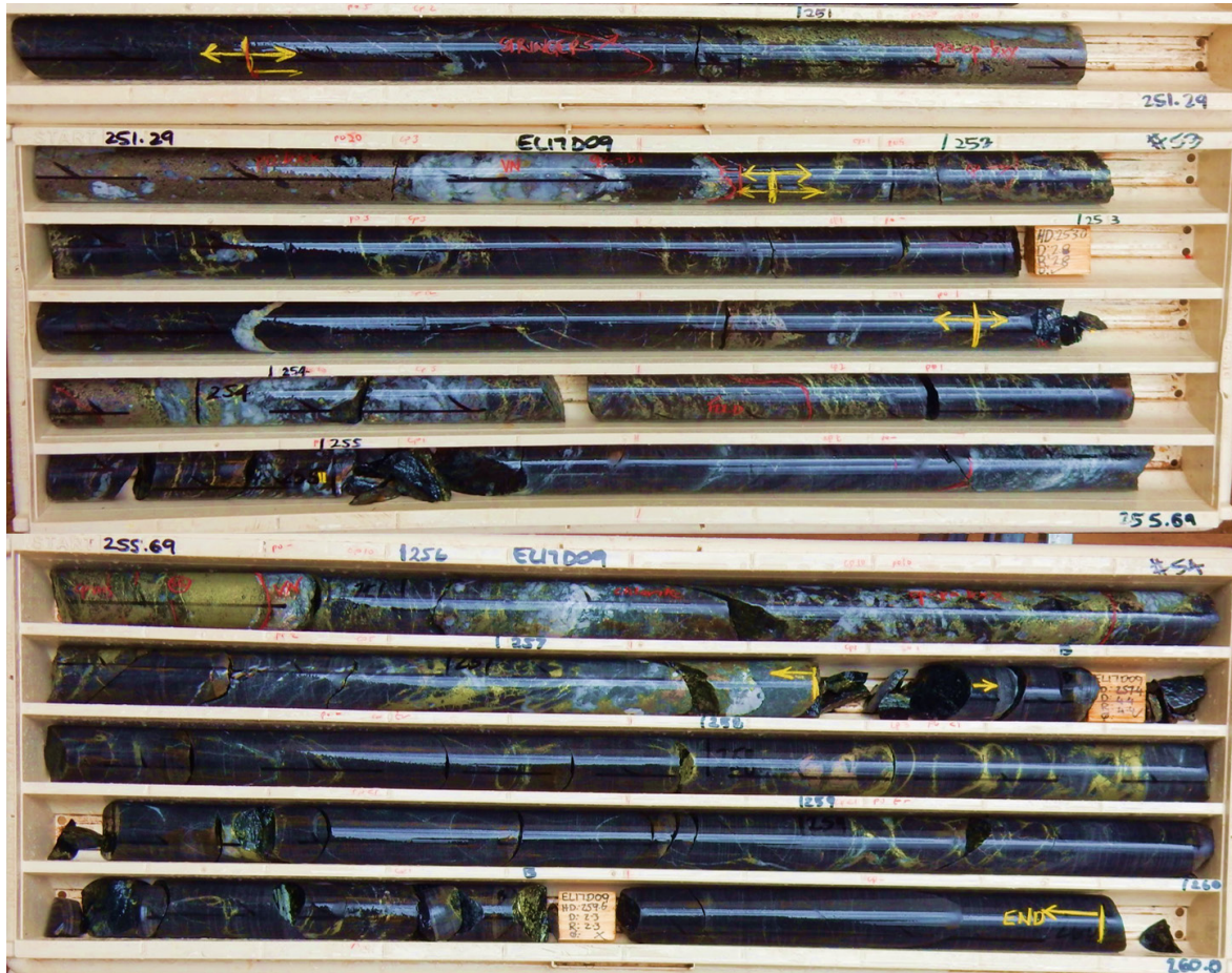
Figure 6: EL17D09: zone of strong copper sulphide mineralisation at J1 position between 251-259.6m. Chalcopyrite is yellow, pyrrhotite is bronze in colour
